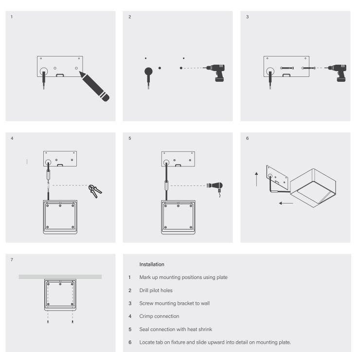
7 Screw fixture to mounting plate
